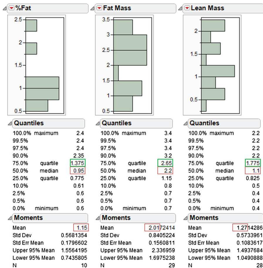
Fig. 7. Histograms and statistical analyses of precision data from Table 2 for percent fat, fat mass and lean mass. The 75th percentile values were taken as an indicator for establishing the recommended performance expectations of 2% for percent fat, 3% for fat mass, and 3% for lean mass.
